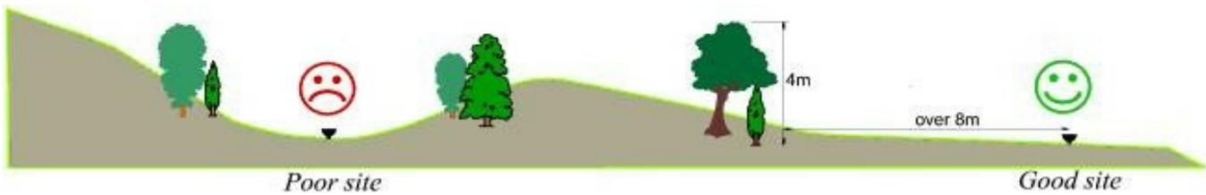
The rain sensor should, ideally, be situated at a distance of twice the height of local obstructions and mounted 30cm (12") above ground level. This requirement can often be difficult or impossible to achieve due to surrounding bushes, trees etc. For most practical purposes accuracy will not be greatly impaired if the site is only a distance equal to the height of the obstructions.
